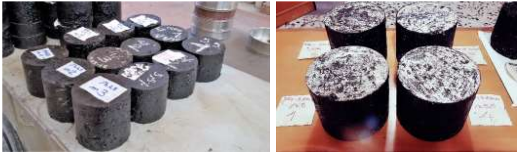
Figure 20. Compacted SGC Specimens of HMA_RFI 15x12cm and DRY mixtures
