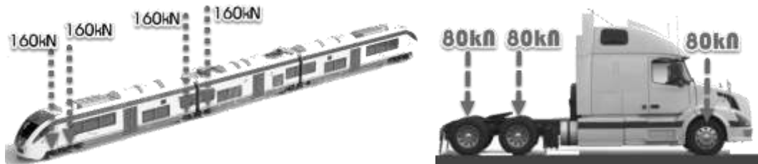
Fig. 4. (a) Convoy Aln 501- Ale Minuetto (train for simulations); (b) Vehicle considered for road simulations
